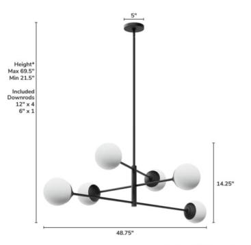
\*Height is ceiling to bottom of fixture
