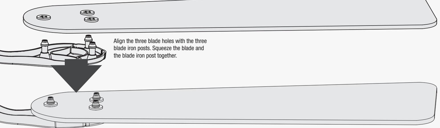
Align the three blade holes with the three blade iron posts. Squeeze the blade and the blade iron post together.
