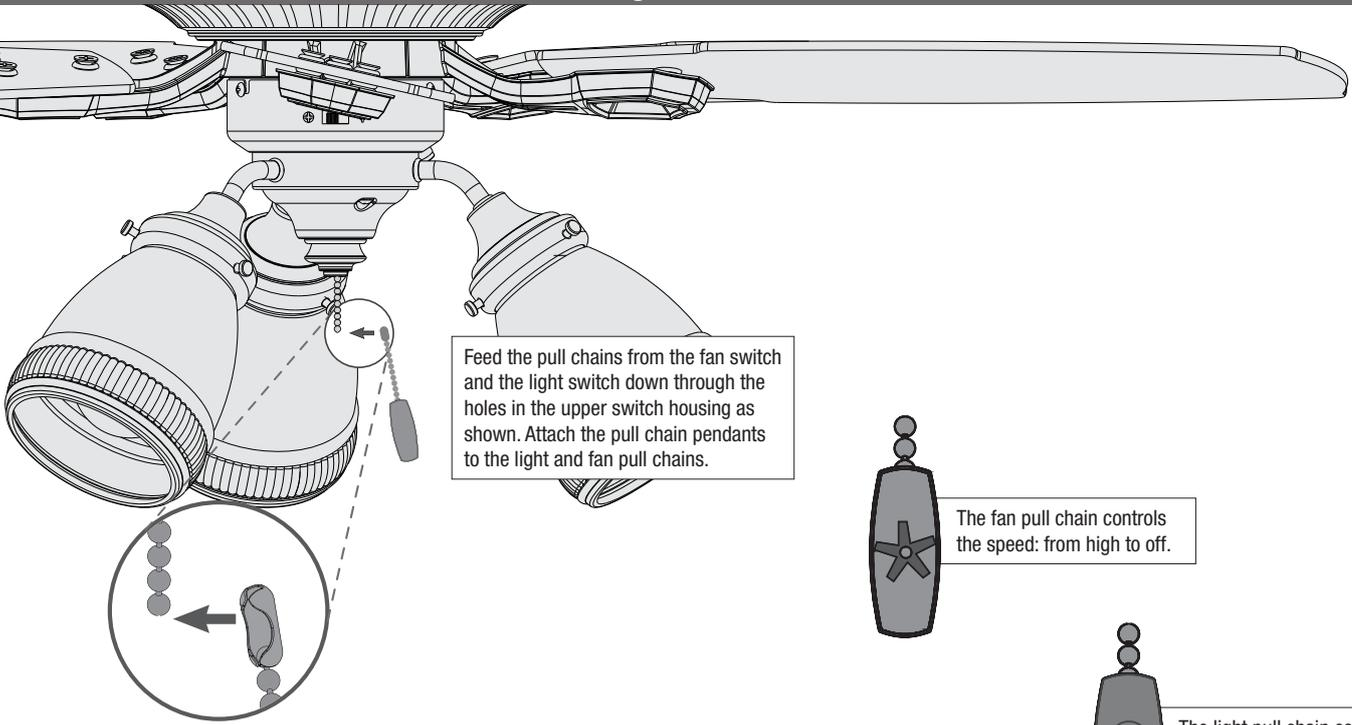
Feed the pull chains from the fan switch and the light switch down through the holes in the upper switch housing as shown. Attach the pull chain pendants to the light and fan pull chains.
