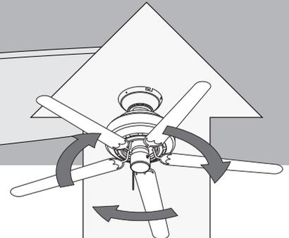
Updraft (clockwise rotation) creates a more indirect airflow. Updraft airflow is great for moving warm air downward.
