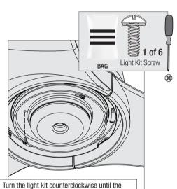
light kit screws are firmly situated in the narrow end of the keyhole slots. Install the third screw and tighten all three screws securely.
