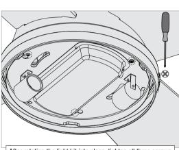
After rotating the light kit into place, tighten all three screws securely.
