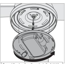
Connect the plugs from the motor to the light kit. Make sure to line up the colored markings on the connectors. Fit light kit keyhole screws onto the three trim ring screws and twist counterclockwise to secure light kit into place.
