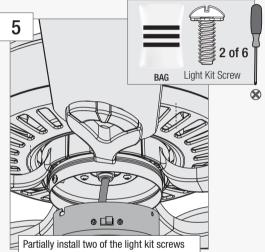
Partially install two of the light kit screws found in the hardware bag. Align the notches in the sides of the lower switch housing with the screws on the upper switch housing. Twist the lower switch housing clockwise to lock into place.
