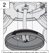
Feed the wire plug through the center hole of the upper switch housing, then wrap keyhole slots around the screws and twist counterclockwise.
