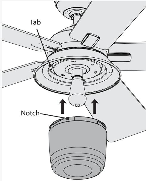
Position the notches in the outer rim of the globe so they line up with the tabs on the light kit assembly. Carefully lift the globe up inside the light kit assembly as far as it will go. Rotate the globe in a clockwise direction until it is held tightly in place by the three tabs.
