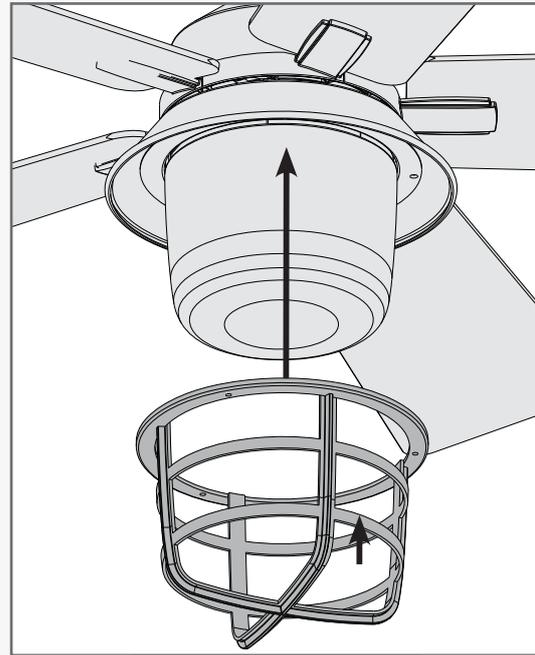
Lift the cage assembly into place
