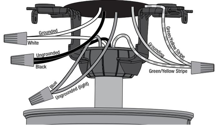
1. Connect the three grounding wires (green, green/yellow stripe, or bare copper) coming from the ceiling, downrod, and hanging bracket.
