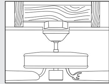
You must be able to secure the fan to building structure or fan-rated outlet box.
