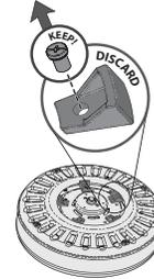
Remove the shipping blocks from the motor. Save the screws. They will be needed for blade iron installation.
