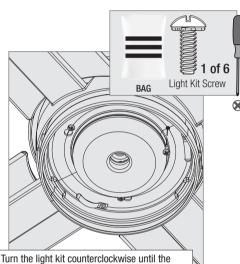
light kit screws are firmly situated in the narrow end of the keyhole slots. Install the third screw and tighten all three screws securely.
