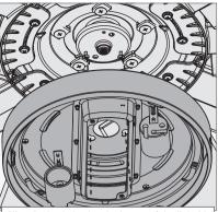
Align the keyhole slots in the top of the light kit assembly with the partially installed assembly screws. Wrap the keyhole slots around the screws and twist counterclockwise.
