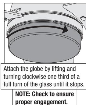
Attach the globe by lifting and turning clockwise one third of a full turn of the glass until it stops.
