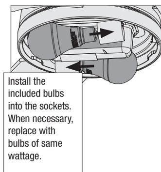
Install the included bulbs into the sockets. When necessary, replace with bulbs of same wattage.
