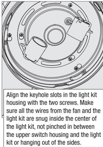
Align the keyhole slots in the light kit housing with the two screws. Make sure all the wires from the fan and the light kit are snug inside the center of the light kit, not pinched in between the upper switch housing and the light kit or hanging out of the sides.
