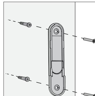
If you are installing into drywall, drill two 9/64 width holes using the cradle bracket as a guide. Gently hammer the included drywall anchors into the pre-drilled holes.
