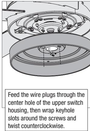
Feed the wire plugs through the center hole of the upper switch housing, then wrap keyhole slots around the screws and twist counterclockwise.
