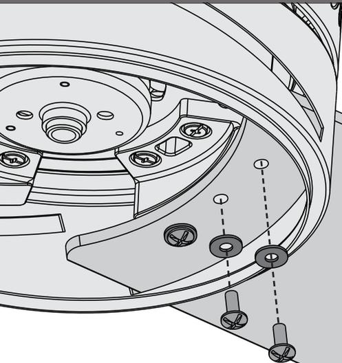
Attach each blade to a blade iron using the blade washers, found in the ■ hardware bag, and the blade assembly screws, found in the ▲ hardware bag.
