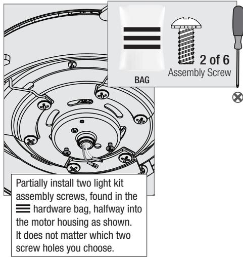
Partially install two light kit assembly screws, found in the hardware bag, halfway into the motor housing as shown. It does not matter which two screw holes you choose.
