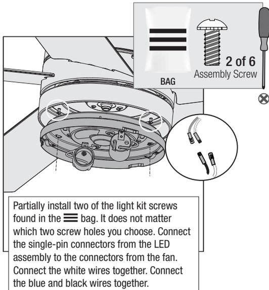
Partially install two of the light kit screws found in the hardware bag. It does not matter which two screw holes you choose. Connect the single-pin connectors from the LED assembly to the connectors from the fan. Connect the white wires together. Connect the blue and black wires together.
