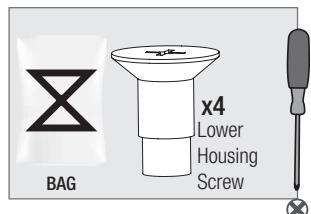
There are four holes on the motor. Lift the lower housing and align the grommet holes in the lower housing with the holes of the motor. It does not matter which hole you choose. Install the lower housing screws found in the hardware bag X to secure the lower housing to the fan.
