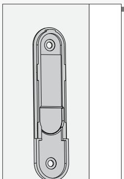
Press the cradle bracket against the wall and hold firmly for 30 seconds.
