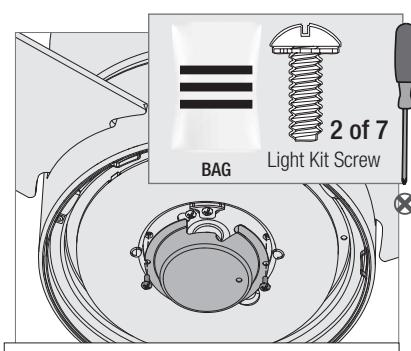
Raise the LED assembly to the trim ring. Align the screw holes in the LED assembly with the screw holes in the trim ring. Screw two light kit assembly screws, found in the hardware bag, through the LED assembly and into the trim ring.
