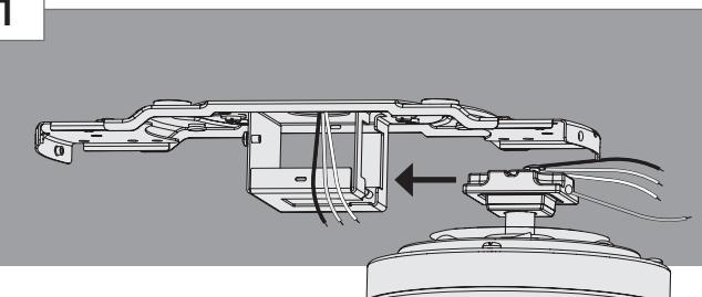
While holding the wires out of the way, lift the motor assembly and place the square hanger into the opening in the ceiling bracket. Be sure the ground wire attached to the hanger faces out of the large opening in the ceiling bracket.
