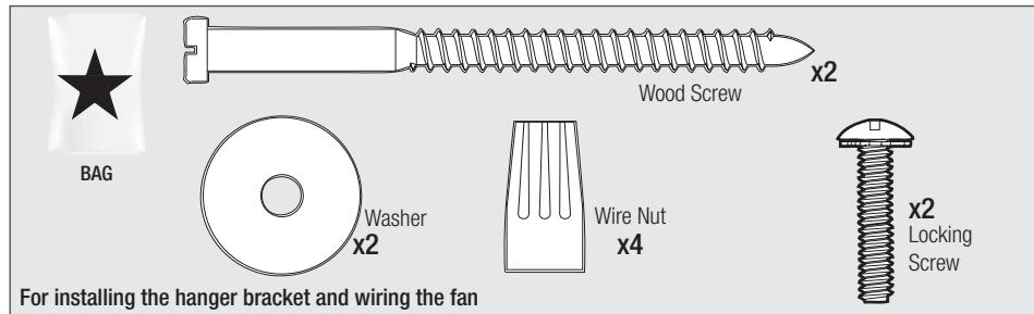
For installing the hanger bracket and wiring the fan
