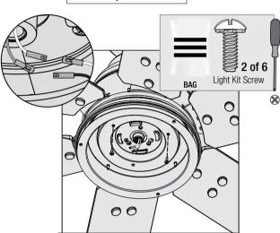
Partially install two of the light kit screws found in \( \equiv \) the bag. It does not matter which two screw holes you choose. Connect the plugs from the upper switch housing and the LED assembly. Make sure to line up the colored markings on the connectors.
