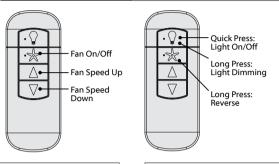
The Fan On/Off button turns the fan on or off. Adjust the fan speed using the "Fan Speed Up" or "Fan Speed Down" directional buttons.
