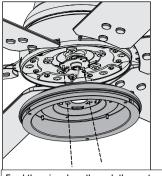
Feed the wire plugs through the center hole of the upper switch housing, then wrap keyhole slots around the screws and twist counterclockwise.
