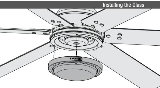
Lift the glass assembly and align the three screw holes of the light kit with the three preassembled thumbscrews of the glass assembly. Tighten all three thumbscrews to secure.
