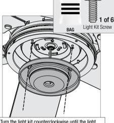
Turn the light kit counterclockwise until the light kit screws are firmly situated in the narrow end of the keyhole slots. Install the third screw and tighten all three screws securely.
