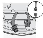
Connect 9-pin to the plug connector found in the switch housing area of the light kit assembly. Make sure to line up the colored markings on the connectors.
