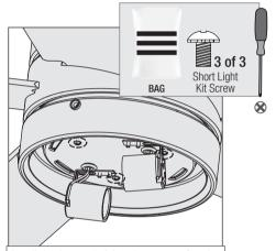
Install the three switch housing screws, found in the hardware bag  $\blacksquare$  . Tighten all three screws.
