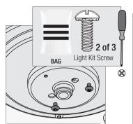
Partially install two light kit assembly screws, found in the hardware bag, halfway into the motor housing as shown. It does not matter which two screw holes you choose.
