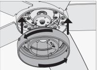
Feed the wire plug through the center hole of the upper switch housing, then wrap keyhole slots around the screws and twist counterclockwise.
