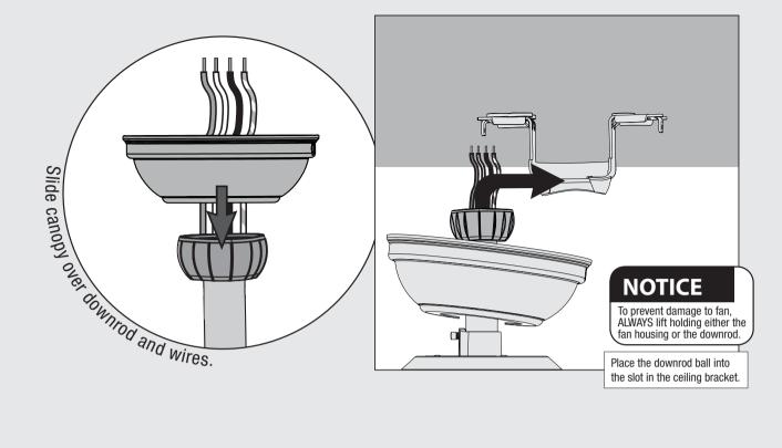
5 Ceiling Bracket Downrod Hanging Fan Wiring Canopy Blades Light Glass/Bulbs
