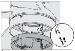
Connect the single-pin connectors from the light kit to the connectors from the fan. Connect the white wires together. Connect the blue and black wires together. Make sure all the wires from the fan and the light kit are snug inside the center of the light kit, not pinched in between the upper switch housing and the light kit or hanging out of the sides.
