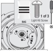
Insert the third screw, found in the hardware bag, into place and then tighten all three screws.
