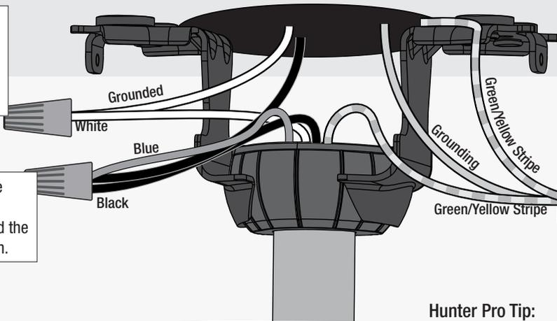
Connect the black wire (ungrounded) from the ceiling to the black and the blue wires from the fan.
