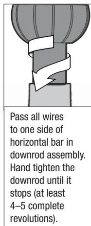
Pass all wires to one side of horizontal bar in downrod assembly. Hand tighten the downrod until it stops (at least 4-5 complete revolutions).
