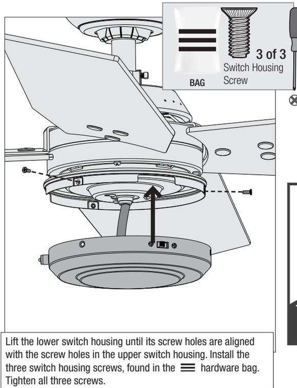
Lift the lower switch housing until its screw holes are aligned with the screw holes in the upper switch housing. Install the three switch housing screws, found in the hardware bag. Tighten all three screws.
