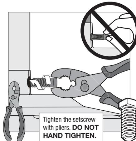
Tighten the setscrew with pliers. **DO NOT HAND TIGHTEN.**
