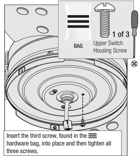
Insert the third screw, found in the hardware bag, into place and then tighten all three screws.
