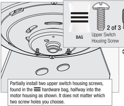
Partially install two upper switch housing screws, found in the hardware bag, halfway into the motor housing as shown. It does not matter which two screw holes you choose.
