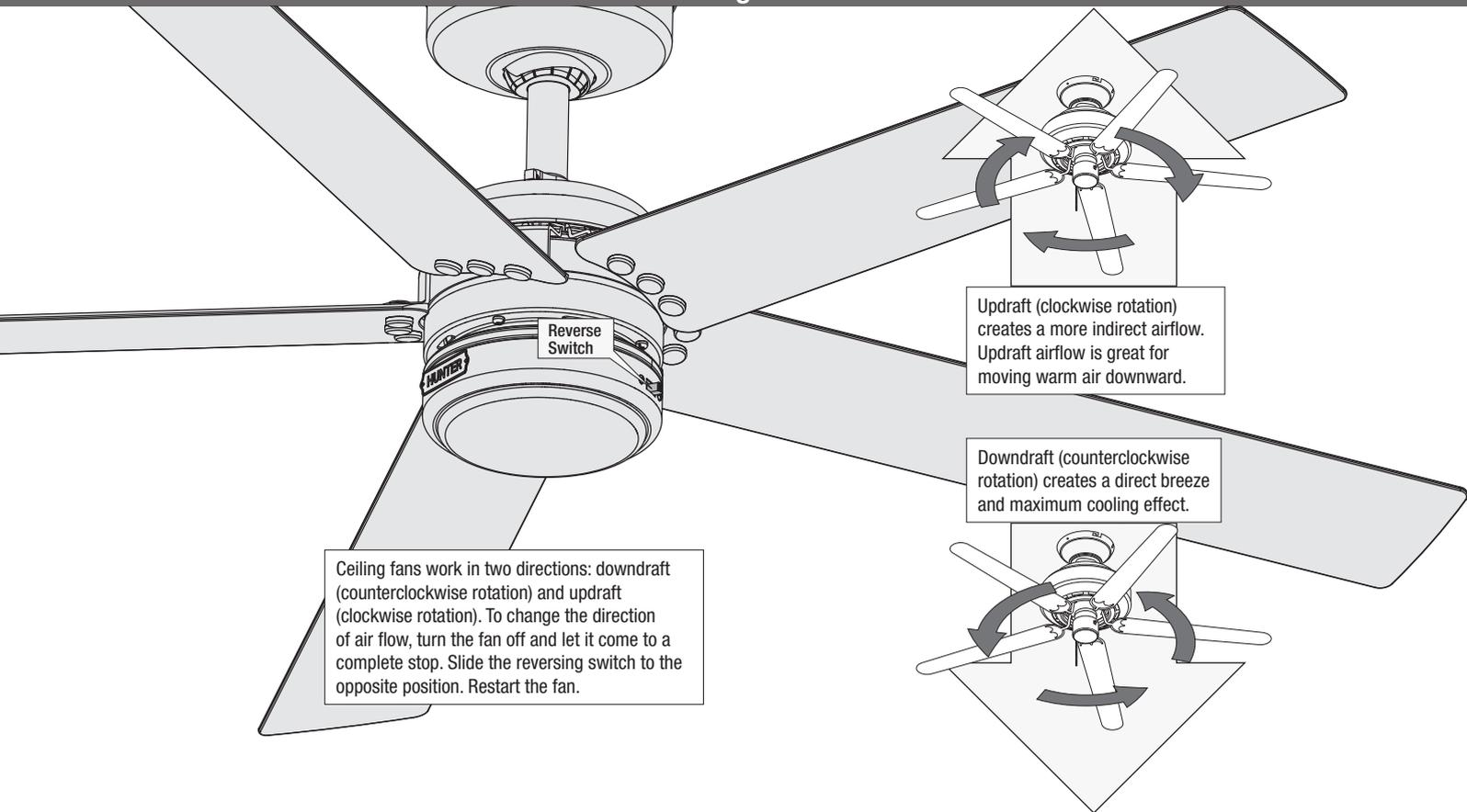
Ceiling fans work in two directions: downdraft (counterclockwise rotation) and updraft (clockwise rotation). To change the direction of air flow, turn the fan off and let it come to a complete stop. Slide the reversing switch to the opposite position. Restart the fan.
