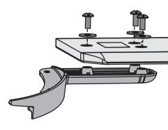
Put the blade washers, found in the hardware bag, onto the blade screws, found in the  $\triangle$  hardware bag. Then install the blade screws to secure each blade to a blade iron.
