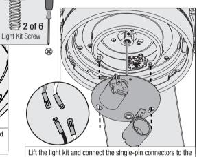
connectors from the fan. Connect the white wires together. Connect the blue and black wires together. Align the keyhole slots in the light kit housing with the two screws. Make sure all the wires from the fan and the light kit are snug inside the center of the light kit, not pinched in between the upper switch housing and the light kit or hanging out of the sides.
