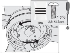
Turn the light kit counterclockwise until the light kit screws are firmly situated in the narrow end of the keyhole slots. Install the third screw and tighten all three screws securely.
