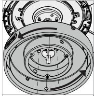
Feed the wire plug through the center hole of the upper switch housing, then wrap keyhole slots around the screws and twist counterclockwise.
