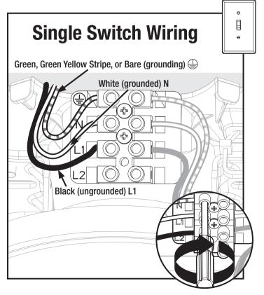
Connect wiring from ceiling to terminal block (on side of canopy mount) and tighten using flathead screwdriver (included).
