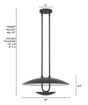
\*Height is ceiling to bottom of fixture
