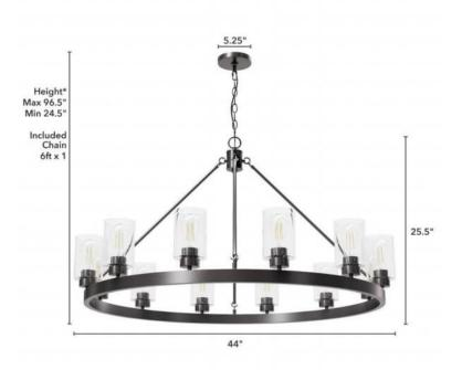
\*Height is ceiling to bottom of fixture
