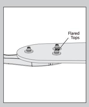
The flared tops of the blade iron posts will be fully visible above the blade when properly assembled.
