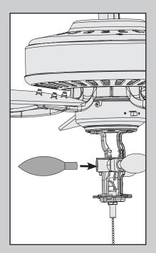
Install a bulb into each of the sockets. When necessary, replace with bulbs of the same type and wattage.
