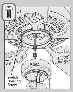
Partially install two of the switch housing screws found in the ≡ bag. Connect the plugs from the upper and lower switch housings. Make sure to line up the colored markings on the connectors.
