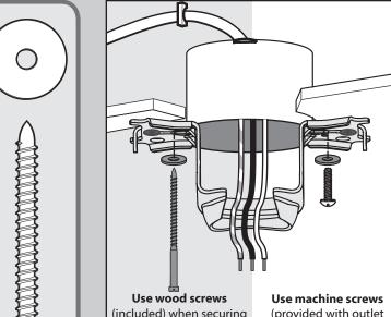
(included) when securing to support structure with approved electrical outlet box. Drill 9/64" pilot holes in support structure to aid in securing ceiling bracket with hardware found in the ★ hardware bag.
