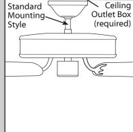
Use **Standard Mounting** or **Low-Profile Mounting** to hang the fan from a flat ceiling.
