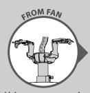
Using an orange wire connector from the  $\bigstar$  hardware bag, connect the 3 grounding wires (green, green/ yellow stripe, or bare copper) coming from the ceiling, downrod, and
