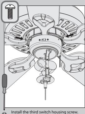
Tighten all three screws securely.
