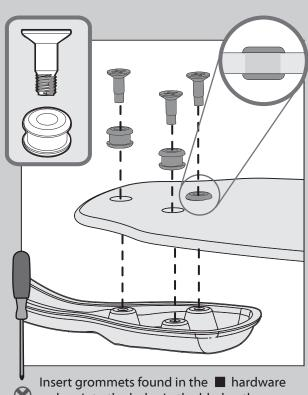
nsert grommets found in the ■ hardware bag into the holes in the blades, then secure each blade to a blade iron with screws found in the ▲ hardware bag.
