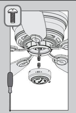
Partially install two of the switch housing screws found in the ≡ bag. Connect the plugs from the upper and lower switch housings. Make sure to line up the colored markings on the plug connectors.
