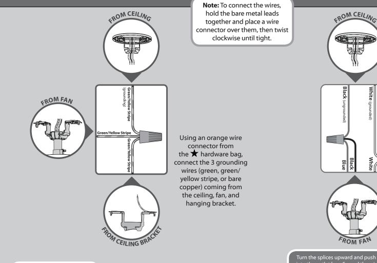
Using the orange wire connectors from the  $\bigstar$  hardware bag, connect the black wire (ungrounded) from the ceiling to the black and the blue wires from the fan. Connect the white wire (grounded) from the ceiling to the white wire from the fan.
