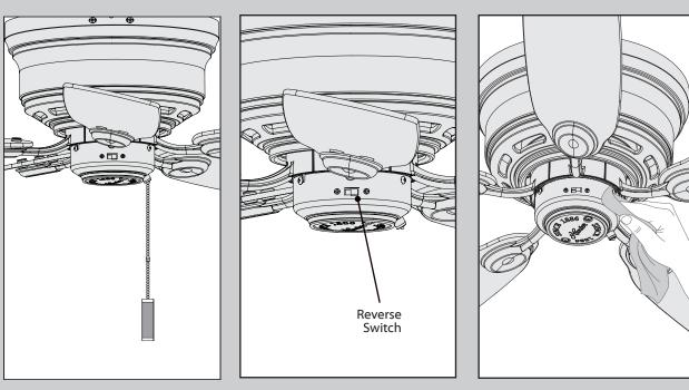
The pull chain controls the fan: from high to off. **Changing the direction of air flow** - move the reverse switch to the opposite position. **Cleaning the fan** - use soft brushes or cloths to prevent scratching. Cleaning products may damage the finishes.
