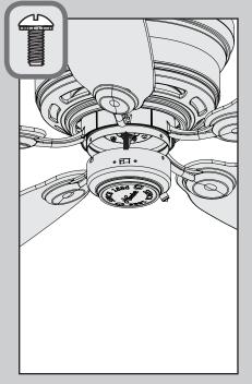
Align the notches in the sides of the lower switch housing with the screws on the upper switch housing. Twist the lower switch housing clockwise to lock into place. Install the third switch housing screw. Tighten all three screws securely.
