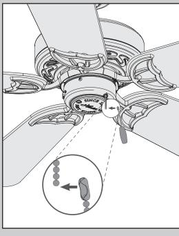
Attach the pull chain pendant to the short chain coming from the switch housing.
