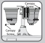
Push the two canopy halves from the kit together around the hanging system. Make sure that the receiver is tucked inside. Partially install the canopy screws from the kit into the screw holes. Slide the canopy up close to the ceiling. Tighten all four screws.
