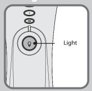
Ouickly press the Light button to turnthe lights off and on. Hold the Light button to raise and dim the light level.
