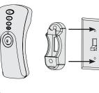
remove the two screws holding your switch cover plate. Do not remove the cover plate. Orient the cradle by lining up the two mounting holes with those on the cover plate. Insert and tighten the screws. Do not over tighten.
