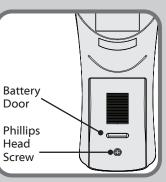
Installing or changing the battery To access the battery compartment remove the small Phillips head screw that secures the battery door to the transmitter assembly. Replace with a CR2032 battery when necessary. The battery should be installed with the positive (+) side up.
