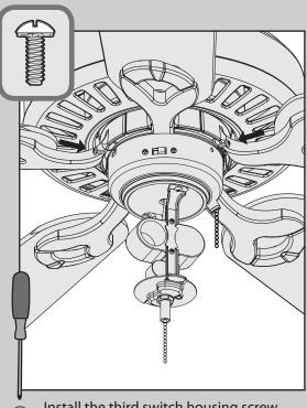
Install the third switch housing screw.
