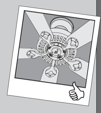
Lightly attach the blade irons to the motor with the blade iron armature screws, then securely tighten after both screws are attached.
