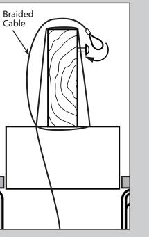
Tighten the loop and secure the screw and washer all the way down to the support brace. Coil up the excess cable.
