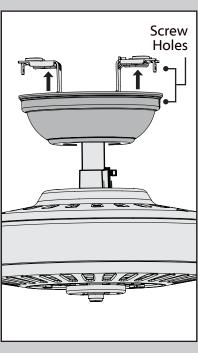
Lift the canopy into place so that the screw holes are aligned.
