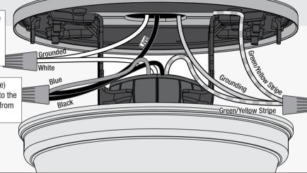
Connect the three grounding wires (green, green/vellow stripe, or bare copper) coming from the ceiling, downrod, and hanging bracket.
