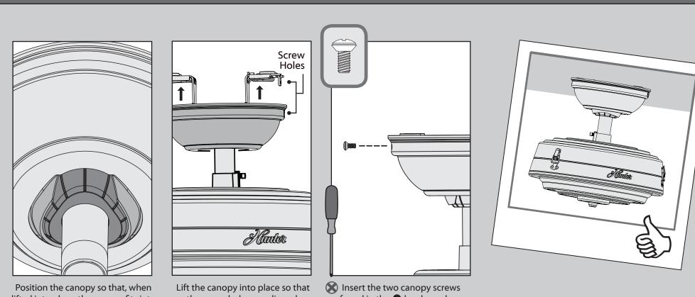
lifted into place, the canopy fits into the hanging bracket as shown.
