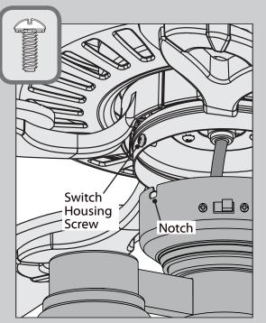
Partially install two of the switch housing screws found in the  $\equiv$  hardware bag. Align the notches in the sides of the lower switch housing with the screws on the upper switch housing. Twist the lower switch housing clockwise to lock into place.
