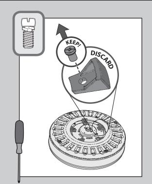
Remove the shipping blocks from the motor. Save the screws. They will be needed for blade iron installation.
