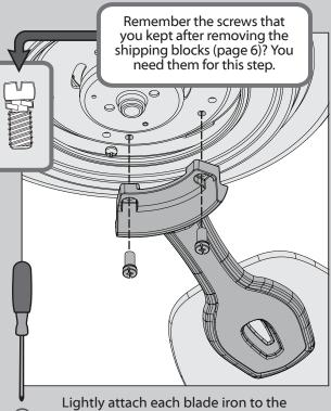
Lightly attach each blade iron to the motor housing with the blade iron armature screws. Securely tighten after both screws are attached.
