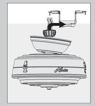
**DO NOT PICK THE FAN UP BY THE CANOPY OR WIRES.** Place the downrod ball into the slot in the ceiling bracket.
