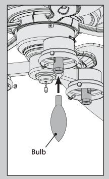
Install a bulb into each of the sockets. When necessary, replace with bulbs of the same type and wattage. To install each shade, first loosen the thumbscrews. Carefully raise the shade to the light fixture and tighten all thumbscrews securely.
