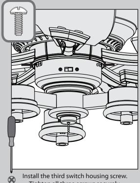
Tighten all three screws securely.
