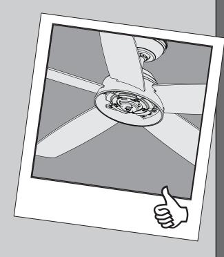
Attach each blade to a blade iron using three blade washers, found in the hardware bag, and three blade assembly screws, found in the hardware bag.
