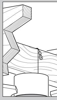
Tighten the loop and secure the screw and washer all the way down to the support brace. Coil up the excess cable.
