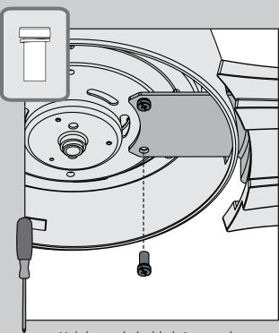
Lightly attach the blade irons to the motor with screws found in the X hardware bag, then securely tighten after both screws are attached. Repeat this step for each blade assembly.
