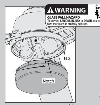
Position the notches in the outer rim of the globe so they line up with the tabs on the inside surface of the light fixture rim.
