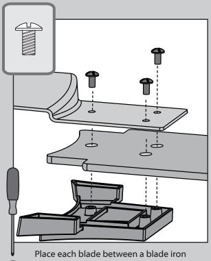
and medallion. Install three blade screws, found in the A hardware bag, to attach the medallion to the blade iron. Repeat this step for each blade.
