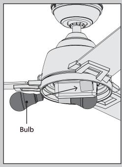
Install a light bulb in each socket. When necessary, replace with bulbs of the same wattage.
