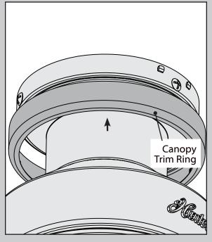
Using both hands, push the canopy trim ring up to the top of the canopy. The canopy trim ring will snap and lock into place.
