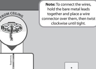
Using an orange wire connector from the ★ hardware bag, connect the grounding wires (green, green/ yellow stripe, or bare copper) coming from the ceiling and ceiling plate.
