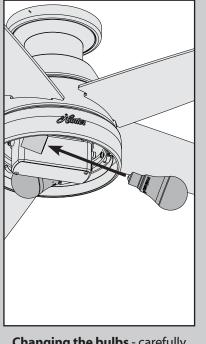
**Changing the bulbs** - carefully remove the globe. Unscrew the bulbs and replace them with bulbs of the same wattage. Reinstall the globe.
