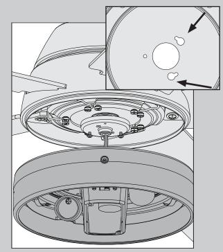
Align the keyhole slots in the top of the light kit assembly with the partially installed assembly screws. Wrap the keyhole slots around the screws and twist counterclockwise.
