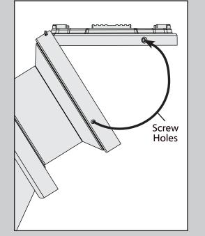
Swing the fan up to align the canopy screw holes with the mounting holes on the ceiling plate.
