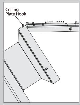
Place the slots over the ceiling plate hooks to hang the fan.
