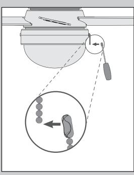
Remove and discard the plastic connectors from the ends of the short pull chain. Connect the appropriate pull chain pendant to each of the short chains. The fan pull chain controls the speed: from high to off. The light pull chain controls the light fixture: on and off.
