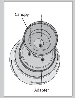
Place the canopy on the top housing. Ensure all four screw holes line up with the screw holes in both the top housing and the adapter.
