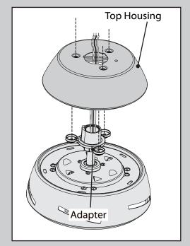
Thread the wires through the top housing. Place the top housing onto the motor housing so that the holes in the top housing lineup with the holes in the motor housing and the adapter.
