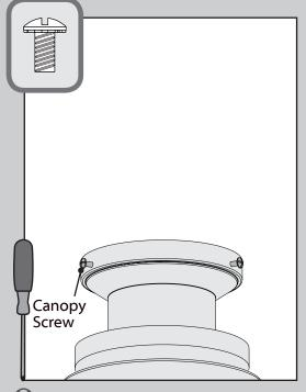
★ Hold the canopy up with the screw holes aligned. Partially install two canopy screws, found in the ● hardware bag, into the holes opposite the ceiling plate hooks.
