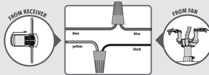
**6 Wiring the receiver and fan to the ceiling**
