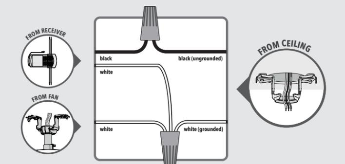
**⚠** Turn the splices upward and push them carefully back through the hanger bracket into the outlet box. Spread the wires apart, with the grounded wires on one side of the outlet box and the ungrounded wires on the other side of the outlet box.
