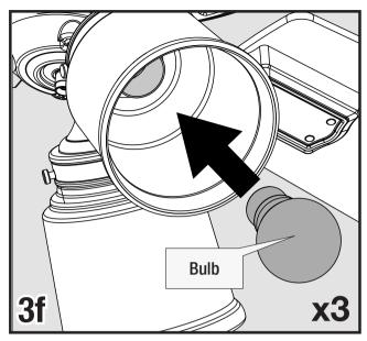
Install a bulb into each of the sockets. When necessary, replace with bulbs of same wattage.
