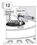
Push the retention spring to the side to allow cross pin access. Place cross pin through downrod assembly and the pivot bracket. Place retention spring into the groove of the cross pin.
