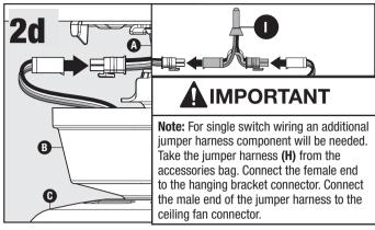
Connect wiring harness from canopy mount ( $\mathbf{A}$ ) to wiring harness from fan body ( $\mathbf{C}$ ).
