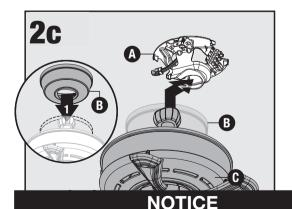
To prevent damage to fan, **ALWAYS** lift holding either the fan housing or the downrod. Do not lift by wires.
