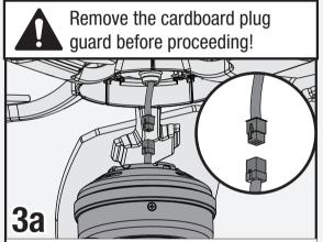
Connect the plugs from the fan and light fixture. Make sure to line up the colored markings on the connectors.
