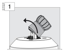
In order to change the length of downrod, the pivot assembly needs to be disengaged. Rotate the downrod into an upright position.
