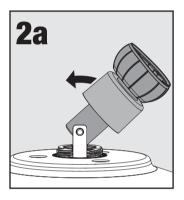
Rotate the downrod into an upright position.
