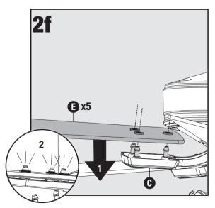
Install a snap-on blade to pop locks on pre-installed blade iron. Repeat for remaining blades (**E**).
