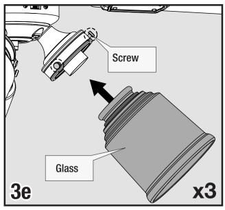
To install the glass, first loosen the thumb screws. Raise the glass to the light fixture. Tighten all thumbscrews securely.
