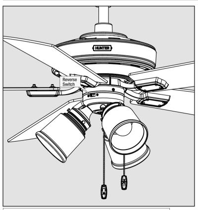
Ceiling fans work in two directions: downdraft (counterclockwise rotation) and updraft (clockwise rotation). To change the direction of air flow, turn the fan off and let it come to a complete stop. The reversing switch is located inside the light fixture. It can only be accessed when the glass is removed. Slide the reversing switch to the opposite position. Restart the fan.
