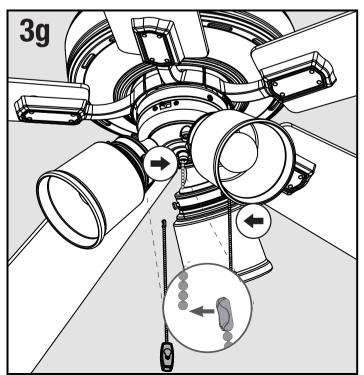
Attach the pull chain pendants to the light and fan pull chains.
