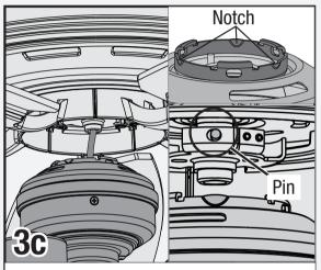
Raise the light kit to the bottom of the fan. Align the notch on the mounting ring on the top of the light kit with the pin in the mounting bracket on the bottom of the fan.
