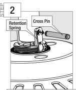
Disengage retention spring by pulling away from rod. Then remove cross pin from downrod. Remove downrod assembly from pivot assembly.
