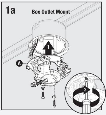
Install canopy mount (A) to box outlet. Secure with machine screws and washers (provided with outlet box).
