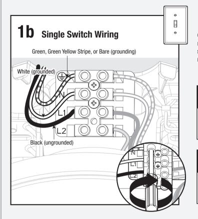
Connect wiring from ceiling to terminal block (on side of canopy mount) and tighten using flathead screwdriver (included). For single switch wiring an additional jumper harness component will be needed which is seen in step 2d.
