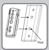
Your Universal Remote comes with a wall plate that has two (2) posts on which to mount your transmitter when not in use.
