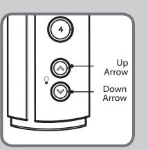
The up arrow and down arrow buttons control the lights on the fan. Quickly press the up or down arrow to turn the lights off and on. Hold the up or down arrow to raise and dim the light level.
