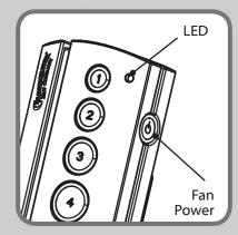
The power button found on the right side of the transmitter turns the fan off. The LED light will illuminate when a button is pushed, letting you know that the signal has been sent to the fan.
