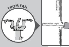
Using an orange wire connector from the \* hardware bag, connect the three grounding wires (green, green/yellow stripe, or bare copper) coming from the ceiling, downrod, and hanging
