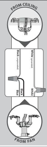
Using orange wire connectors from the  $\bigstar$  hardware bag, connect the black wire (ungrounded) from the ceiling to the black and the blue wires from the fan. Connect the white wire (grounded) from the ceiling to the white wire from the fan.
