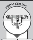
Note: To connect the wires, hold the bare metal leads together and place a wire connector over them, then twist clockwise until tight.
