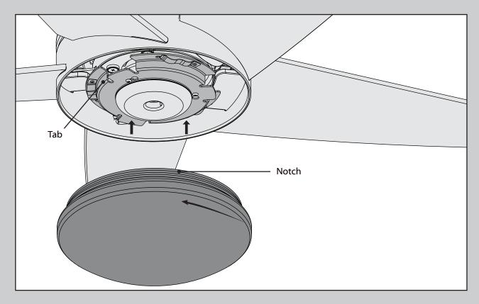
Align the notches in the globe assembly with the tabs in the light kit fitter. Carefully lift the globe assembly as far as it will go, then rotate it counterclockwise until it is held into place by the three tabs.
