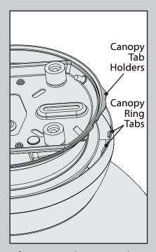
Before going to the next step, locate the two sets of canopy ring tabs that are on the top edge of the canopy and the two sets of canopy tab holders found at the top of the fan body near the ceiling.
