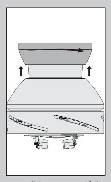
To install the canopy ring, lift the canopy, then rotate clockwise until the tabs are held in place by the tab holders, locking the canopy ring into place.
