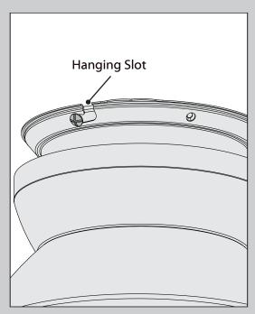
Using both hands, lift the fan body from the hook and align the hanging slots on both sides of the fan body with the two partially installed canopy screws. Slide the two slots on both sides of the fan body between the head of the screws and rotate the fan body clockwise so the screws hold the fan body firmly in place.
