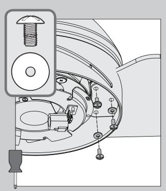
Install the blade using three blade screws and washers, found in the ▲ hardware bag. Repeat this process for all five blades.
