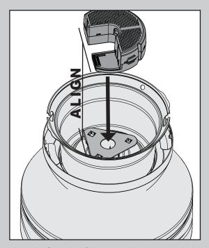
Align the flat side of the control receiver with the flat side of the triangular seat. Lower the control receiver on the triangular seat. Ensure the posts on the bottom of the control receiver are seated in the holes in the triangular seat.
