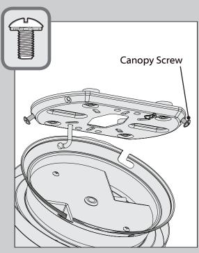
Partially install two of the canopy screws into screw holes on opposite corners of the ceiling plate as shown. Choose the two screw holes that are aligned with the hanging slots in the fan body.
