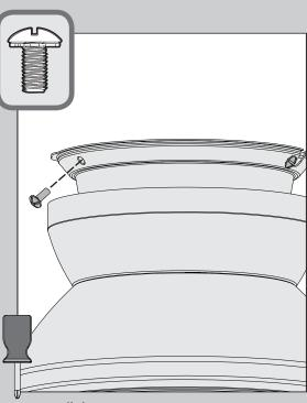
Install the remaining two canopy screws by holding the fan body cover to the ceiling mounting plate. Tighten all four screws securely.
