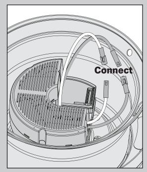
Locate the single-pin connectors that are taped together. Connect the single-pin connectors from the control receiver to the connectors from the fan. Connect the white wires together. Connect the blue wires together. The third, loose wire will not be used for your installation. It is capped to prevent usage.
