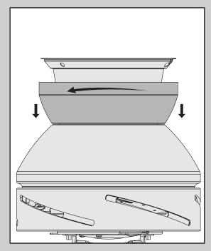
Unlock the canopy cover from the canopy ring tabs to loosen the canopy ring and lower it down to the fan body as shown.
