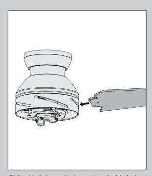
Slide a blade into a slot located on the blade ring.
