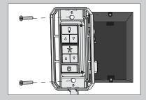
Installing the Wall Plate
