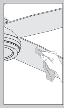
When cleaning the fan, use soft brushes or cloths to prevent scratching. Cleaning products may damage the finishes.
