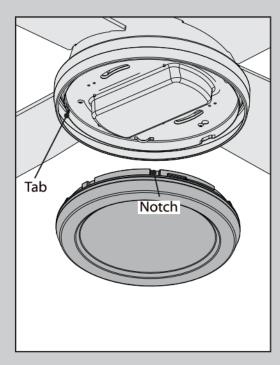
Lift the switch housing cap and align the notches in the globe with the tabs in the switch housing. Attach the cap to the switch housing kit by twisting it clockwise until it snaps into place.
