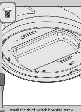
Tighten all three screws securely.
