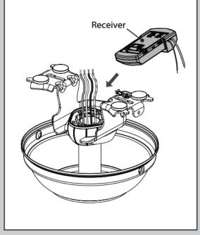
Place the receiver on top of the downrod assembly as shown.
