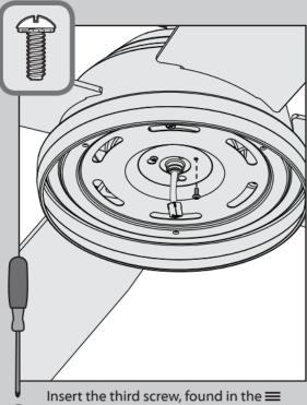
A hardware bag, into place and then tighten all three screws.
