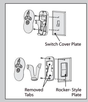
To install the transmitter cradle, remove the two screws holding the switch cover plate. Do not remove the cover plate. Orient the cradle by lining up the two mounting holes with those on the cover plate. Insert and tighten the screws. Do not over tighten.
