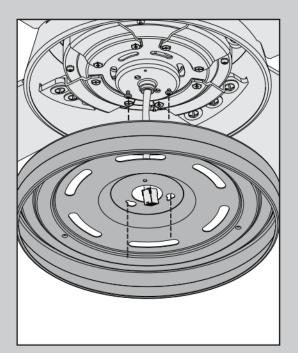
Feed the wire plug through the center hole of the upper switch housing, then wrap keyhole slots around the screws and twist counterclockwise.
