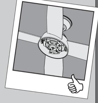
Attach each blade to a blade iron using three blade washers, found in the hardware bag, and three blade assembly screws, found in the  $\triangle$  hardware bag.
