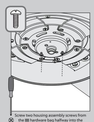
motor housing. It does not matter which
