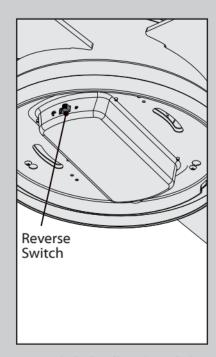
To switch the direction of air flow, move the reverse switch to the opposite position. You will need to remove the glass to do so.
