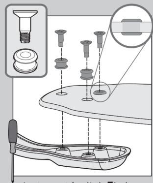
Insert grommets found in the hardware bag into the holes in the blades, then secure each blade to a blade iron with screws found in the  $\triangle$  hardware bag.
