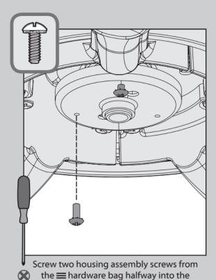
motor housing. It does not matter which
