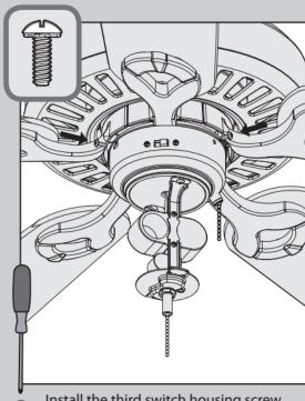
Install the third switch housing screw.
