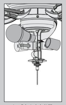
Install the included LED bulbs into the sockets. When necessary, replace with bulbs of same wattage.
