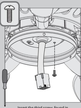
Insert the third screw, found in the = hardware bag, into place and then tighten all three screws.
