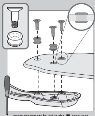
Insert grommets found in the **n** hardware bag into the holes in the blades, then secure each blade to a blade iron with screws found in the **A** hardware bag.
