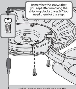
Lightly attach the blade irons to the motor with the blade iron armature screws, then securely tighten after both screws are attached.
