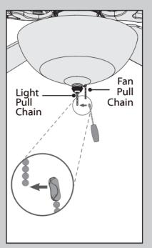
Remove the plastic break away connector. Connect the appropriate pull chain pendant to each of the short chains coming from the finial and finial cap. The fan pull chain controls the speed: from high to off. The light pull chain controls the light fixture: on and off.
