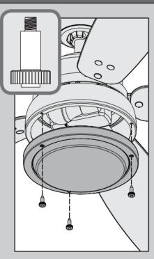
Lift the globe assembly and attach it to the upper switch housing using the three thumbscrews, found in the = hardware bag. Tighten all three screws securely by hand.
