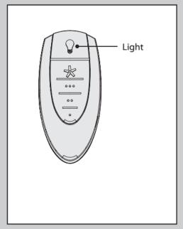
Quickly press the Light button to turn the lights off and on. Hold the Light button to raise and dim the light level.
