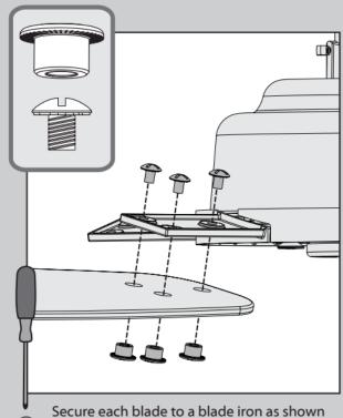
Susing the blade nuts, found in the ■ hardware bag, and the blade assembly screws, found in the **A** hardware bag.
