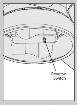
To switch the direction of air flow, remove the globe assembly and move the reverse switch to the opposite position. Reinstall the globe assembly.
