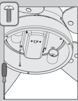
Turn the light kit counterclockwise until the light kit screws are firmly situated in the narrow end of the keyhole slots. Install the third screw and tighten all three screws securely.
