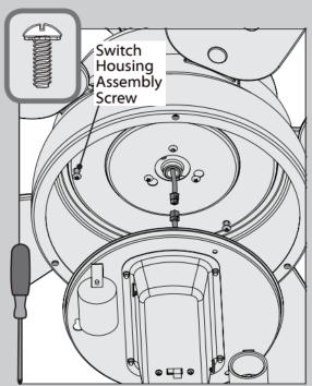
Partially install two of the switch housing assembly screws found in the = bag. It does not matter which two screw holes you choose. Connect the plugs from the upper and lower switch housings. Make sure to line up the colored markings on the connectors.
