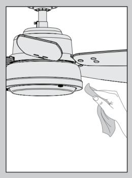
For cleaning the fan, use soft brushes or cloths to prevent scratching. Cleaning products may damage the finishes.
