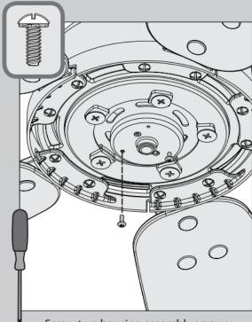
Screw two housing assembly screws from the
