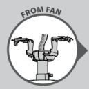
Using an orange wire connector from the  $\bigstar$  hardware bag, connect the 3 grounding wires (green, green/ yellow stripe, or bare copper) coming from the ceiling, downrod, and hanging bracket.
