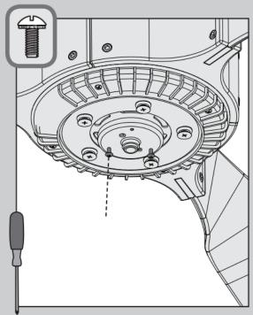
Screw two housing assembly screws from the
