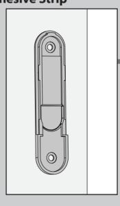
Press the cradle bracket against the wall and hold firmly for 30 seconds.
