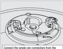
Connect the single-pin connectors from the LED assembly to the connectors from the fan. Connect the white wires together. Connect the blue and black wires together. Tuck the excess wiring above the LED assembly or feed back into the lower switch housing.
