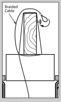
Wrap the braided cable around the support brace once creating a complete circle. Hook the looped end of the cable over the wood screw so that the cable lies between the washer and the support brace.
