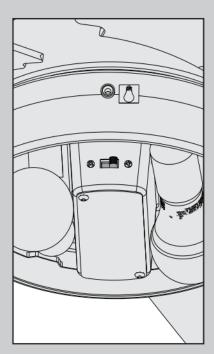
Changing the direction of air flow - carefully remove the globe and move the reverse switch to the opposite position.
