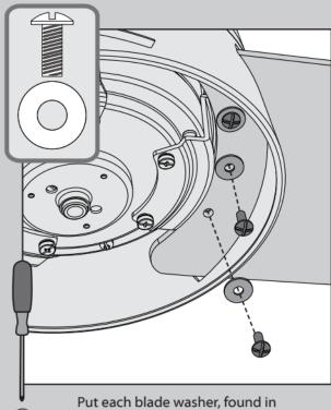
the **n** hardware bag, onto a blade screw, found in the **A** hardware bag. Then secure each blade to a blade iron using the blade screws and washers.
