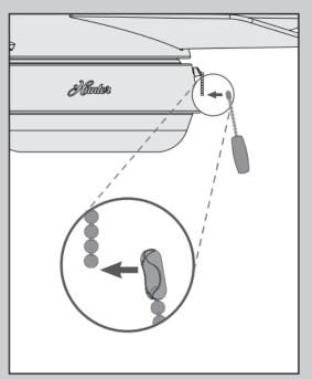
Remove and discard the plastic connectors from the ends of the short pull chain. Connect the appropriate pull chain pendant to each of the short chains. The fan pull chain controls the speed: from high to off. The light pull chain controls the light fixture: on and off.
