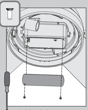
Carefully push all switch housing components into the switch housing, then install the switch housing plate using two light kit assembly screws, found in the
