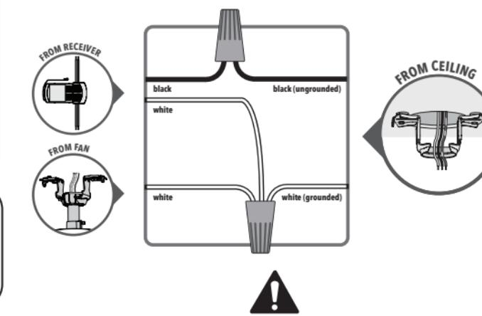
Turn the splices upward and push them carefully back through the hanger bracket into the outlet box. Spread the wires apart, with the grounded wires on one side of the outlet box and the ungrounded wires on the other side of the outlet box.
