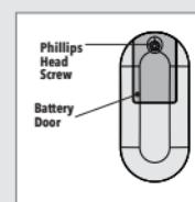
Replace the used battery with a CR2032 battery when necessary. The battery should be installed with the positive (+) side up.
