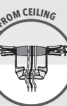
**6 Wiring the receiver and fan to the ceiling**
