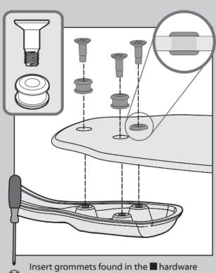
bag into the holes in the lades, then secure each blade to a blade iron with screws found in the lades. hardware bag.
