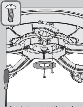
Screw two housing assembly screws from
