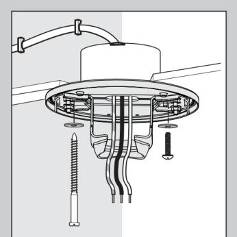
Use wood screws (included) and washers when securing to support structure with approved electrical outlet box. Drill 9/64" pilot holes in support structure to aid in securing ceiling bracket with hardware found in the hardware bag.
