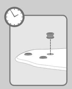
Time Saver Tip: Get a helper to insert grommets, found in the hardware bag, into the blades while you're doing the next couple of steps.
