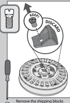
Remove the shipping blocks from the motor. Save the screws. They will be needed for blade iron installation.
