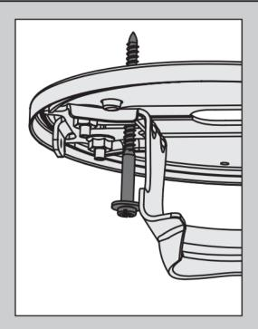
Use the wood screw to poke holes through the rubber gasket in order to install the ceiling bracket assembly to your support structure or ceiling fan-rated outlet box.
