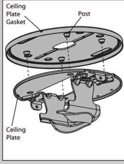
Install the ceiling plate gasket onto the ceiling plate. The four holes in the ceiling plate should lineup with the four posts in the gasket.
