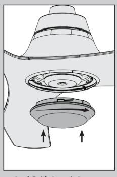
Carefully lift the no-light cap up inside the LED assembly as far as it will go and rotate the cap clockwise until it is held tightly in place by the tabs.
