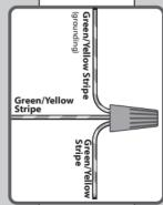
Using an orange wire connector from the hardware bag, connect the three grounding wires (green, green/yellow stripe, or bare copper) coming from the ceiling, downrod, and hanging bracket.
