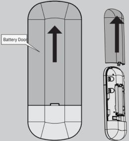
Install two AAA batteries, found in the remote control hardware bag, into the transmitter. Clean the battery contacts prior to installing the batteries. Please contact your local battery recycling center for proper battery disposal information.
