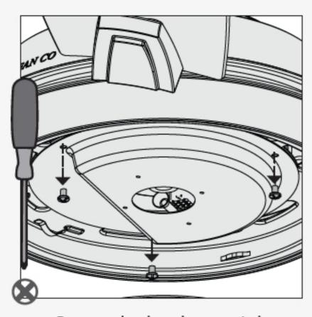
Remove the three lower switch housing screws to remove the lower switch housing. Set aside the components.
