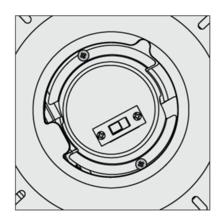
Remove the switch housing cap by removing the two light kit assembly screws. Set aside the components.
